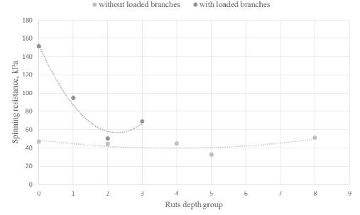
Fig. 3. Shear resistance depending on the technological strip strengthening
